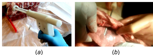
Fig. 3 (a) NTTD prototype test on pork ribs and (b) isolated detection system being tested for safety in porcine tissues
